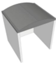
Soffitto a botte Barrel vault ceiling
